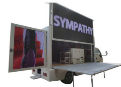
FOTON, Engine : 88hp, LED Screen : Three Sides P8 ( Liftable ) with Hydraulic Stage
