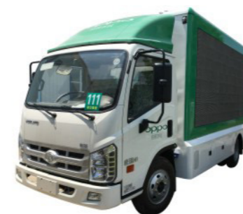
Forland, Engine : 125hp, LED Screen : Double Sides P6 with Banner Roller
