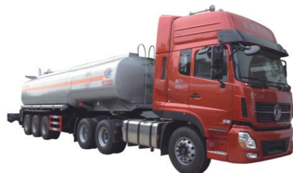
3 axles 48CBM fuel tank semi trailer
