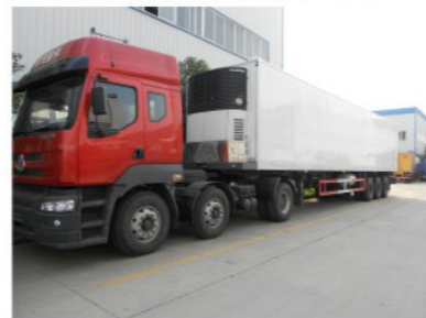
3 axles 40 feet Refrigerator trailer with Carrier units
