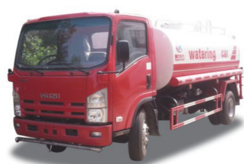
ISUZU water tank truck,engine:ISUZU 190hps, volume:6-8CBM
