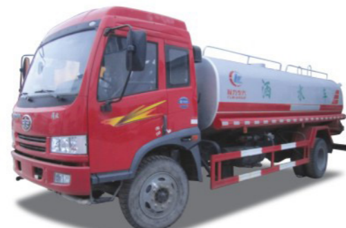
FAW water tank truck, engine:Xichai 180hps, volume:8-10CBM
