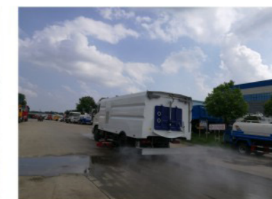
Rear spray water
