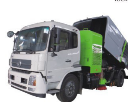
Dongfeng cleaning sweeper truck, 7m3 dust tank & 3.5 water tank
