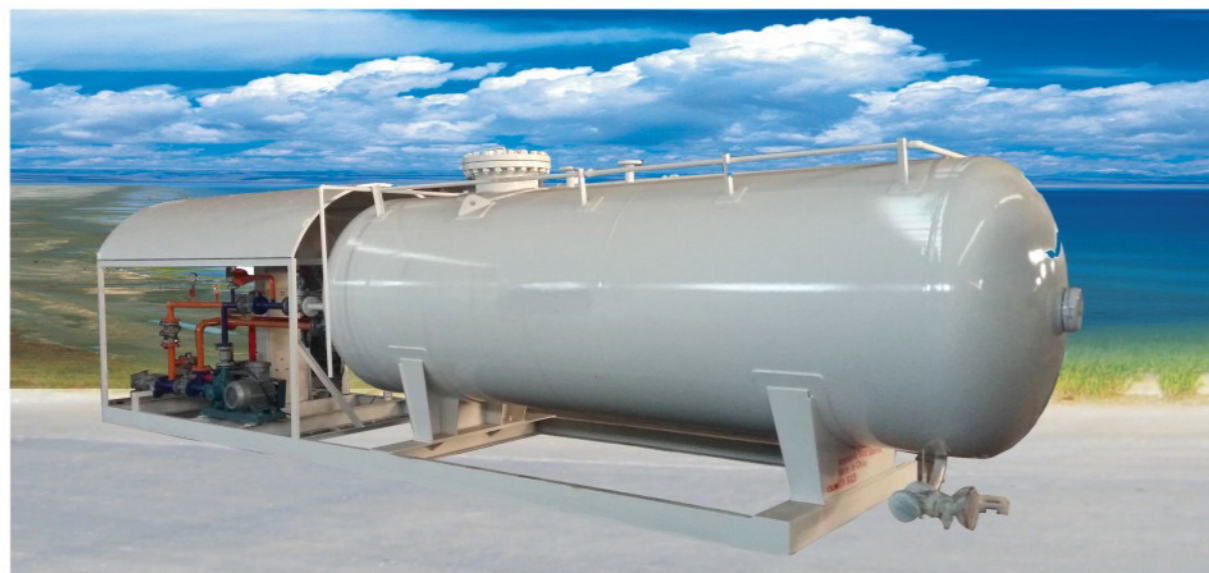
LPG Skid Station Material: Q345R/ASME SA516 Pressure: 1.77Mpa Tank volume: 5CBM-60CBM Medium:Propane/Liquefied Petroleum Gas
