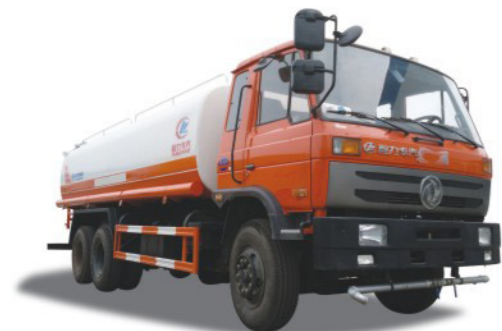
Dongfeng water tank truck, engine:Cummins 210hps, volume:18-20CBM
