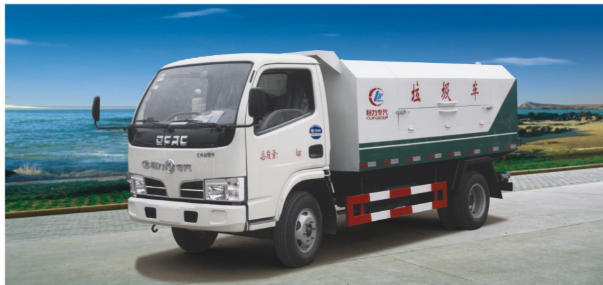
DONGFENG Sealed dump garbage truck, CHAOCHAI engine 95hp,4-5m3
