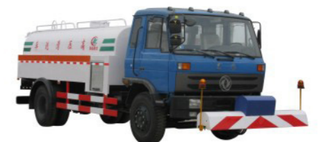
Dongfeng road flushing truck, 8m3 tank, 170hp
