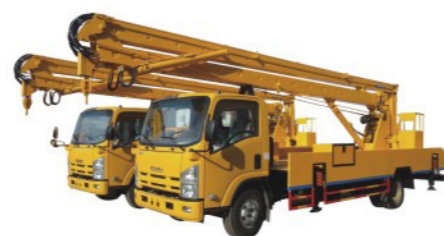
Brand : ISUZU 4*2 LHD Engine: 120HP Working Height :10-16m
