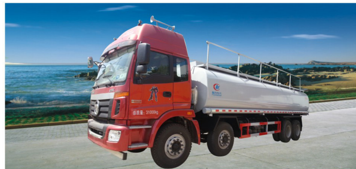
FOTON 8x4 chassis, 290 hp , 30-35cbm fuel tank
